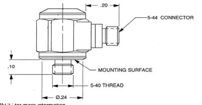
Units on the line drawing are in inches, units in brackets are in millimeters. Refer to 127-3035CG for more information.
